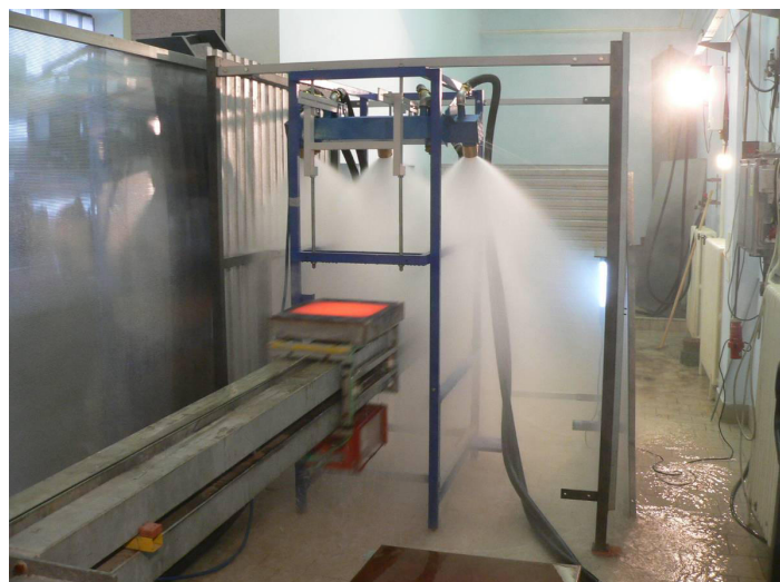
Figure 1. Linear laboratory stand with conic nozzles spraying
