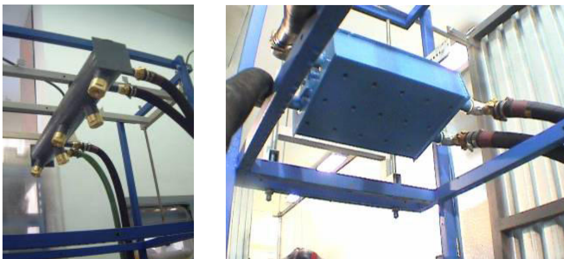
Figure 3. Various types of cooling headers (nozzles and holes)
