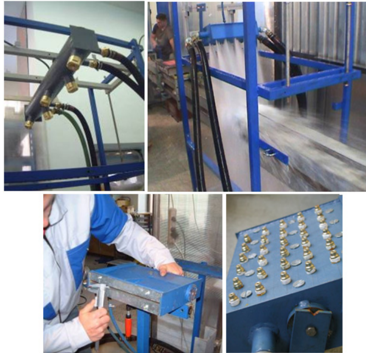
Fig. 2 Various types of cooling headers (full cone nozzles, drilled holes, adjustable slit, cluster of solid jet nozzles)
