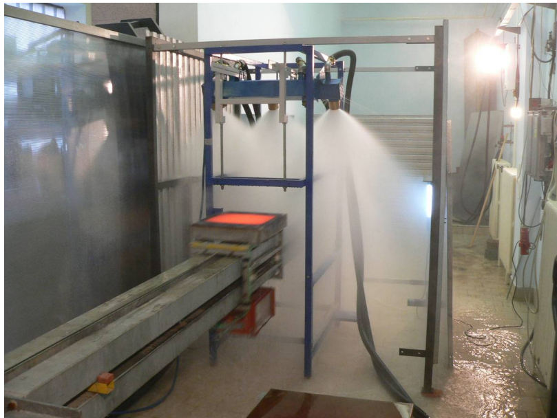
Fig. 1 Linear laboratory stand with test plate moving under group of full cone nozzles
